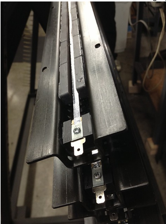
The ribbon within the completed tweeter assembly
